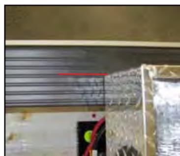
Align the tool box on the left side of the bed with the front lip of the edge liner
