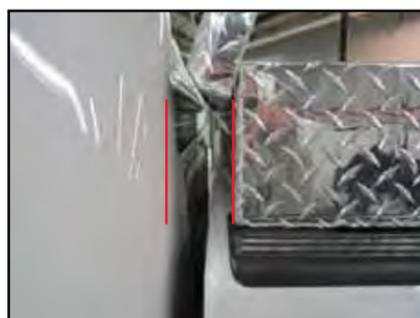
Make sure there is adequate clearance between back of cab and tool box lid when the lid is open
