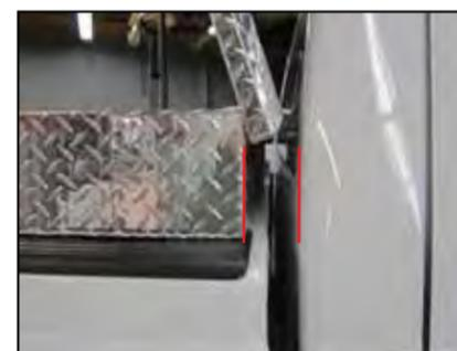
Make sure there is adequate clearance between back of cab and tool box lid when the lid is open
